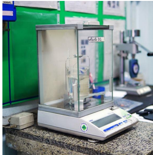
Specific Gravity Tester : SG
