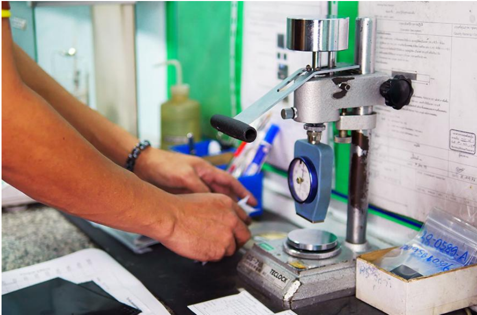
Hardness Tester : Hs
