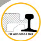
Rubber Railway Level Crossing Panel | External Dimension : 600 x 728 x 170 mm.
